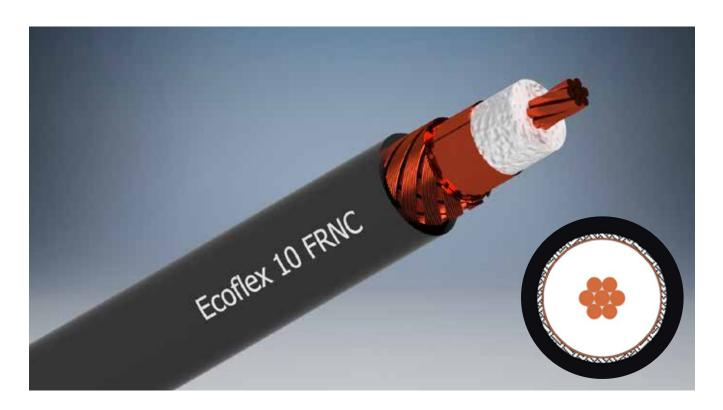
Ecoflex 10 FRNC is a flexible, low loss 50 ohm coaxial cable for the frequency range up to 6 GHz. Advanced manufacturing techniques combined with the use of a low loss PE-LLC dielectric with a foaming rate of more than 70% result in very low attenuation values, which set standards among flexible coaxial cables of this dimension.
